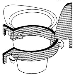
$120^{\circ}$  apart, pass through the ring near the lower edge, directed toward its center, one screw being immediately under the handle. The tips of the screws are bored to admit very short pieces of platinum wire, 1 mm. in diameter, and are then compressed to hold the latter in place. The device weighs approximately 25 grams.
